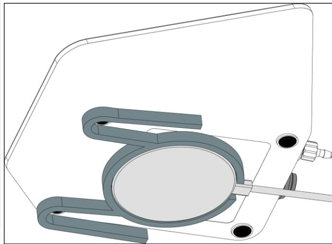
Figure 2. Position of charging plate.
