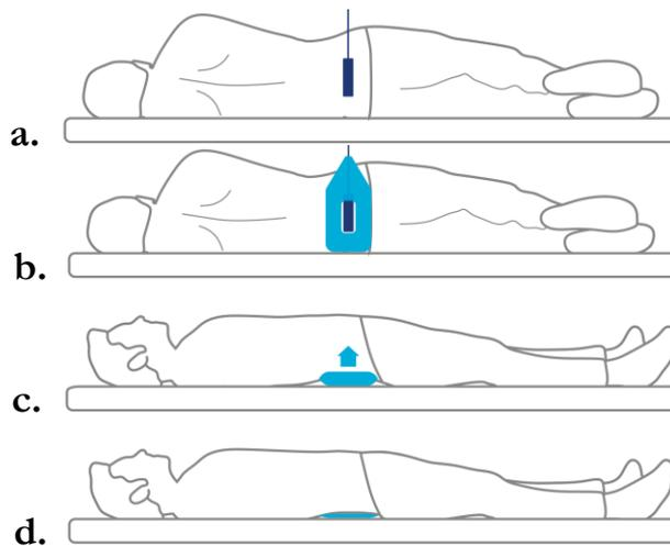
Figure 5. a) Placement of sensor plate. b) Placement of inflatable. c) Inflated inflatable. d) Deflated inflatable.
